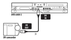
Use a DV cable (not supplied) to connect the DV jack of your DV camcorder/video deck to the front panel DV IN jack of this recorder.
